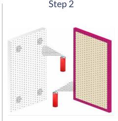
Spray the contact adhesive vertically onto the panels reverse surface and horizontally onto the desired installation area, including the impaling clips. Ensure that 100% of the surface area on both surfaces is covered with the adhesive.
