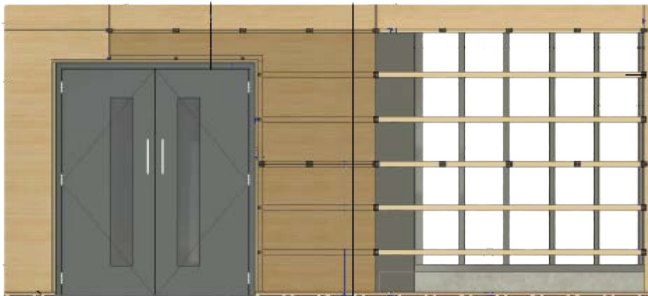
Typical vertical/horizontal studwork construction at 400mm centres to accommodate the installation of the panels.
