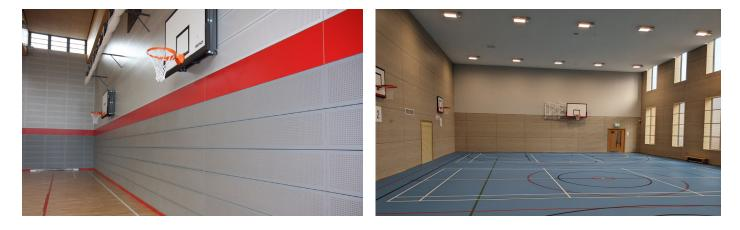
The DYNAMIK Internal Sports Walling panels are both durable, cost effective and provide a highly decorative solution for busy sports hall environments. With high scratch and impact resistance and certified for sport, the panels are designed to be an integral component of the internal wall construction and can be fitted from floor to soffit. Solid panels can be combined with matching or contrasting Class A perforated (acoustic) panels to provide a continuous, flush wall finish.
